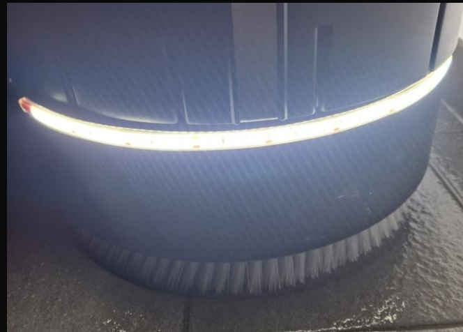
Single-disc prototype: brush and light ring on wet tiles
