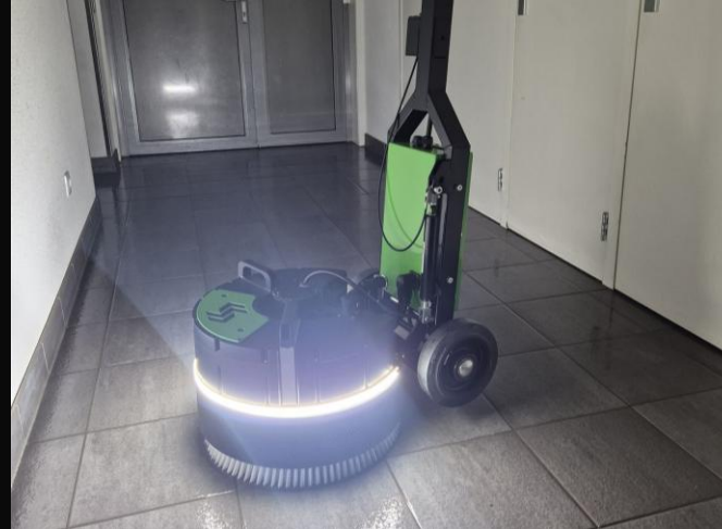
Our second 48 V prototype, a single-disc machine, scrubbing tiles
